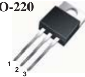
1.Gate 2. Drain 3. Source
